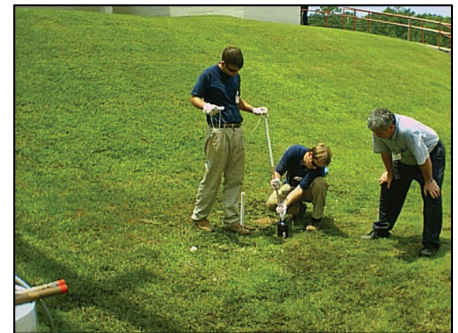
Figure 1. HGS Personnel perform Groundwater Sampling.
